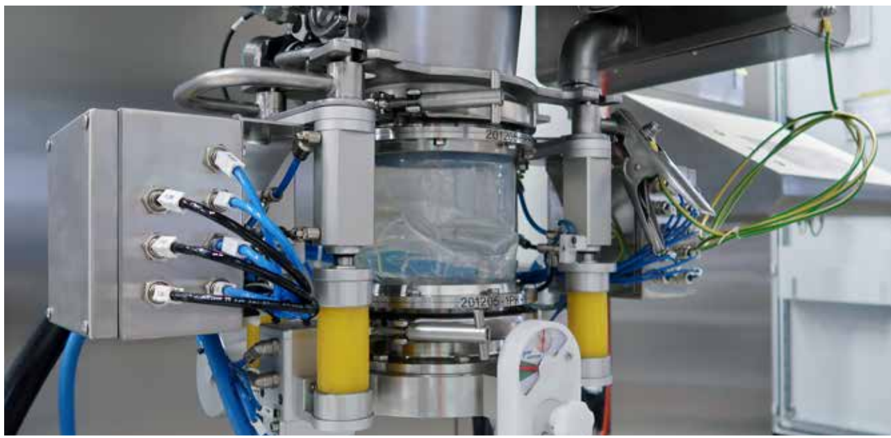
With the containment valves, the VMA ensures secure installation and production in Ex zone 2/22.
